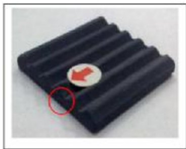
Appearance Description : Crack Failure : More than 2 mm
