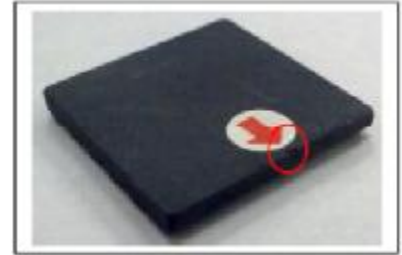
Appearance Description : Hole Limitation : Less than 2 mm
